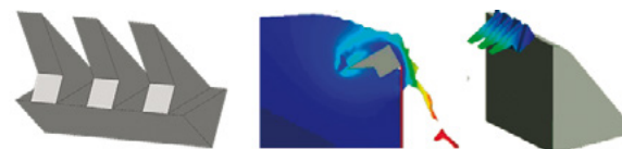
Fuse gates simulation: geometry design (left), fluid-solid interaction 2D simulation (center) and 3D simulation (right)
