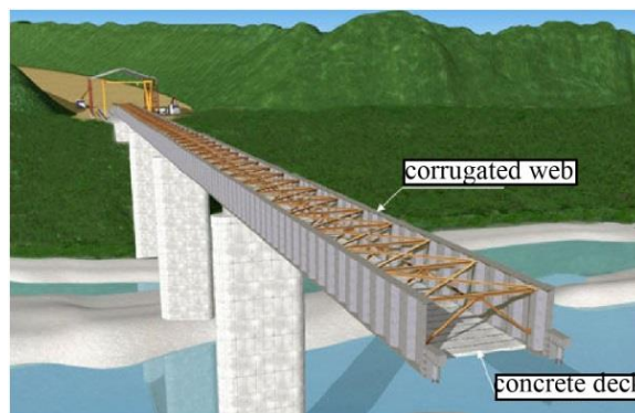
Fig. 1: Example of the launching with corrugate webs
