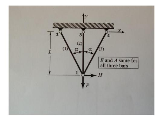
**Part A**: The truss problem is well defined in the figure above, the Elasticity of all bars is E and the area of all bars is A.
