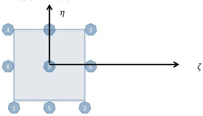
We have a 9-node plane stress element, which it is initially a perfect square. In the before figure we can see the 9 nodes.
