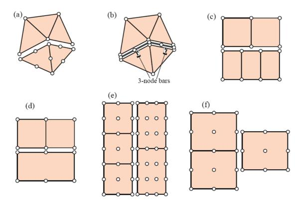
The before meshes fails interelement compatibility:
