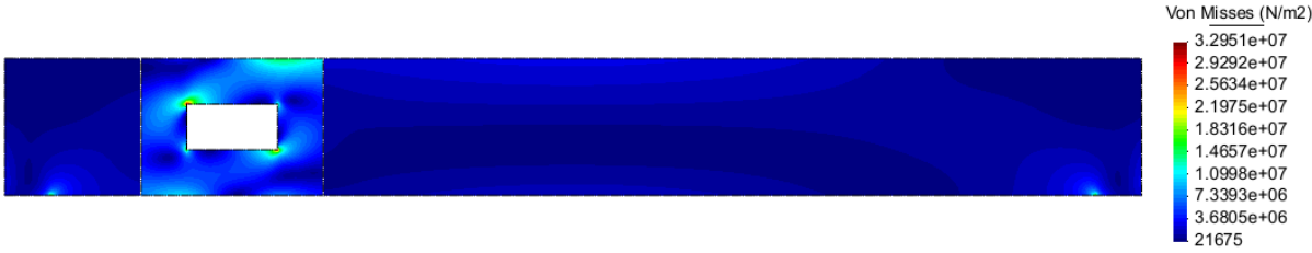
(a) Von Mises stresses for the concrete and steel sections
