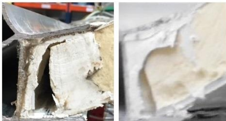
Figure 8.11: State of the adhesive layer after failure during experimental tests performed on model A (left) and model B (right)
