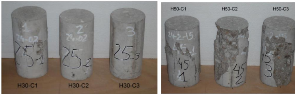
Figure 11: Experimental fracture for concrete samples [64].
