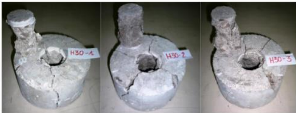
Figure 27: Fractured experimental samples for a H30 concrete in a shear test. [11]
