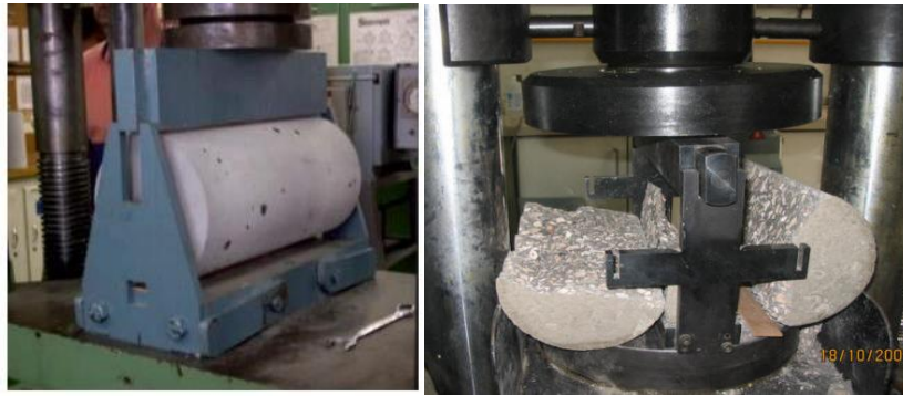
Figure 12: Methodology and fracture of experimental sample in a Brazilian test [18].
