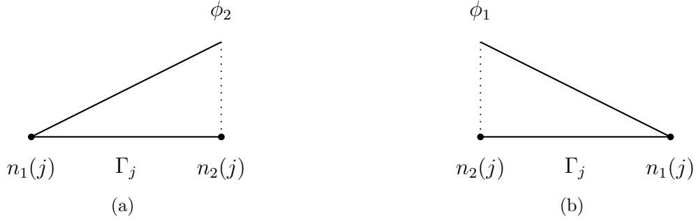
Figure B.1: Two equivalent configurations with different shape functions.
