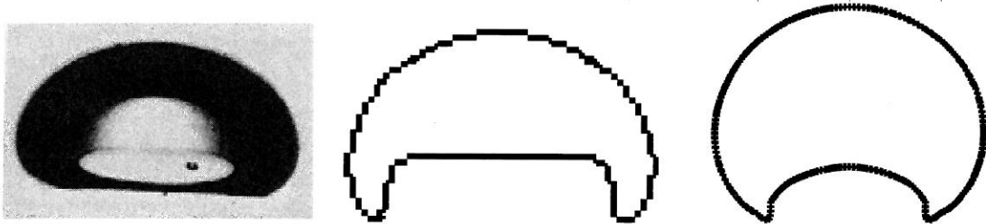
(a) Final bubble shapes of experiments of (Bhaga and Weber, 2007) 1981) (b) Result of (Hua and Lou, 2007) (c) Result of the present code
